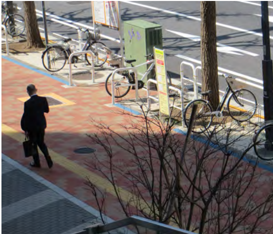
Bike racks, street trees, street lights and utility boxes are all located in a distinctive zone to reduce clutter and maximize pedestrian comfort.
