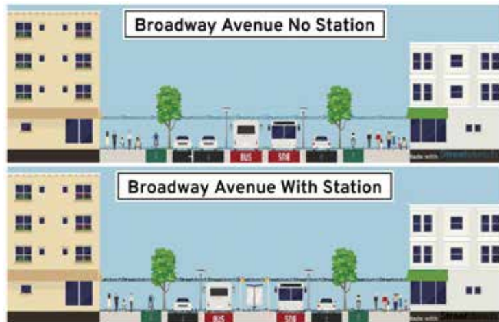
Our vision for Broadway Ave using lessons in traffic calming and prioritization of active and public transportation. Note the buses driving against the flow of traffic (Street Sketch).
